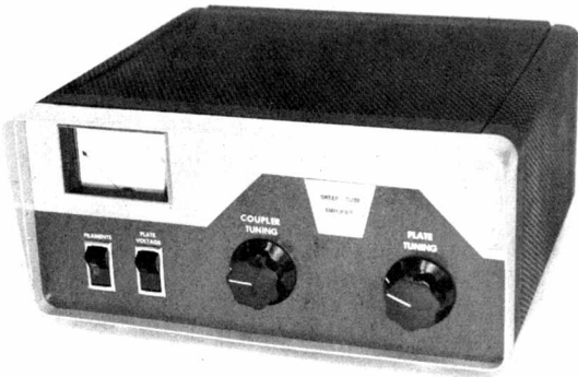
Fig. 1 — Front view of the 800-watt amplifier. An LMB CO-1 cabinet, Simpson 02640 meter, and Kirsh-Kash S-649-70L knobs are used, giving a modern appearance. Coils are changed through the door in the top of the cabinet.
